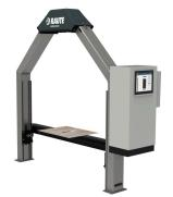
Analyzer with a high-accuracy camera system and industrial light system for optimized veneer dimension and defect detection to control the quality of the veneer sheets going to the gluing process.
