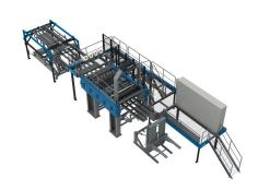
Automate the collection of randoms and compose them into full sheets with strong joints that don't break in drying. Analyzers maximize green veneer recovery.
