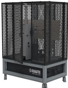
Works as the perfect tool for panel quality control for bending testing, panel stiffness measuring and panel strength measuring
