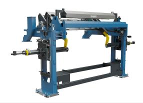
Optimized block centering using laser scanning and autocalibration defines the optimal position to peel out the maximum amount of veneer from each block.
