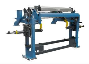
Optimized block centering using laser scanning and autocalibration defines the optimal position to peel out the maximum amount of veneer from each block.
