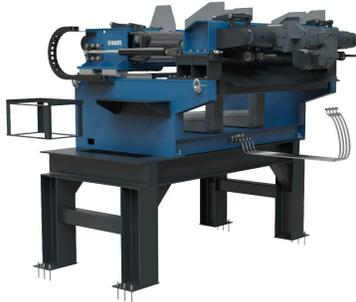
Efficient spindleless debarking and round-up lathe for straight small diameter blocks. Continuous production guaranteed with robust Nordic design.
