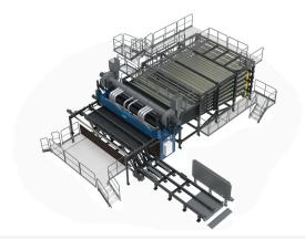
Solid dryer infeed (20 feeds/min) solution with guaranteed performance for full veneer sheets.
