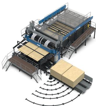
Efficient infeed (24 feeds/min) with all the bells and whistles including random and thin veneer feeding.
