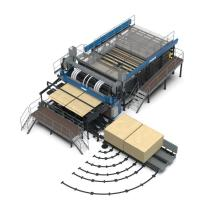
Efficient infeed (24 feeds/min) with all the bells and whistles including random and thin veneer feeding.
