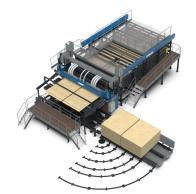
Efficient infeed (24 feeds/min) with all the bells and whistles including random and thin veneer feeding.
