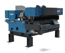
Spindleless, electric peeling lathe that peels highquality veneer from small diameter blocks. Unmatched thickness tolerance with optimal peeling geometry.
