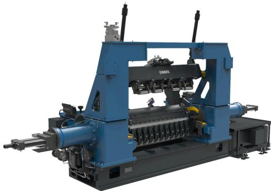
Proven technology with modern optimal peeling geometry. High-quality veneer production from birch and small diameter plantation wood with standard solution.
