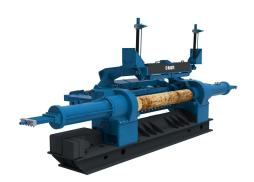
Peel high-quality veneer from all raw materials. Reach maximum capacity through automation and benefit from the flexibility of modular lathe technology.
